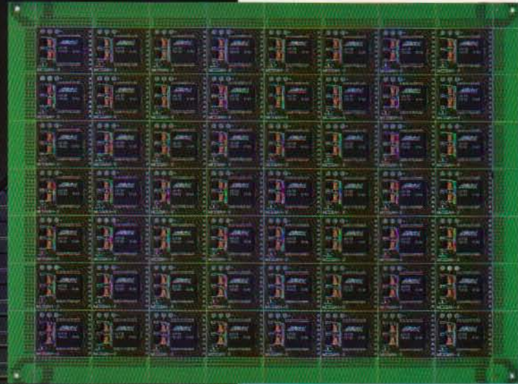
A sheet of newly manufactured mod chips from the Messiah factory in China
